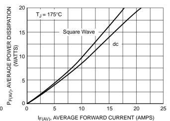
Figure 2. Power Dissipation
