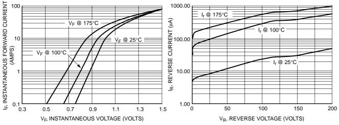
Figure 3. Maximum Forward Voltage
