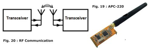
The module's energy consumption is low (+/- 30mA) and installation is rather simple. These features are the basic reasons to choose the module for wireless communictions.
