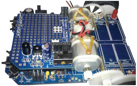
Fig. 6 : ASURO with radio control PCB (Side view)
