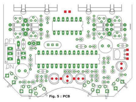
**B.2.** Solder the supplied socket parts on these connection areas. Install the  $1\times3$  socket on the connectors featuring three adjacent areas. The shape of the area is not important. Now you can solder the remaining  $1\times2$  sockets on the free connection areas
