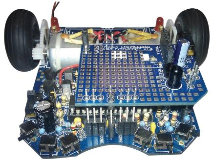
Fig. 7 : ASURO with radio control PCB (Front view)
