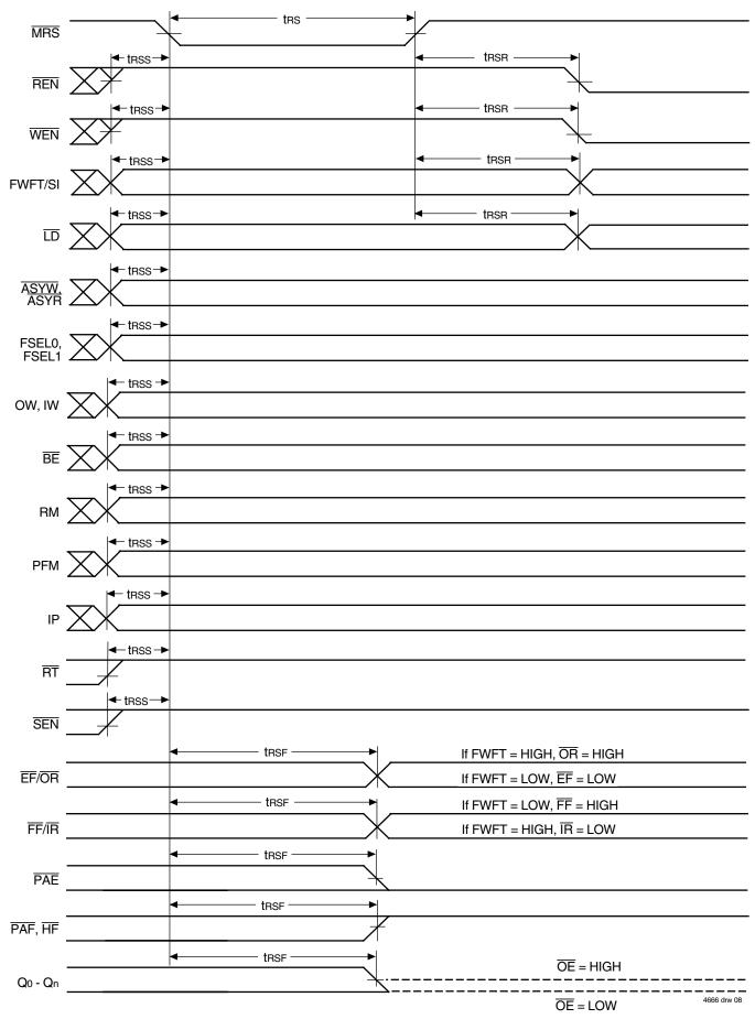
Figure 5. Master Reset Timing
