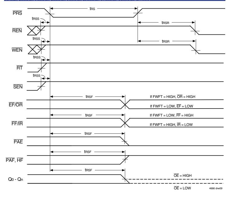
Figure 6. Partial Reset Timing
