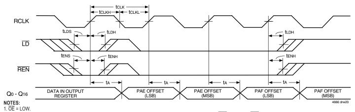
2. This diagram is based on programming the IDT72V293 x18 bus width. Add one extra cycle to both the PAE offset and PAF offset for x9 bus width.
