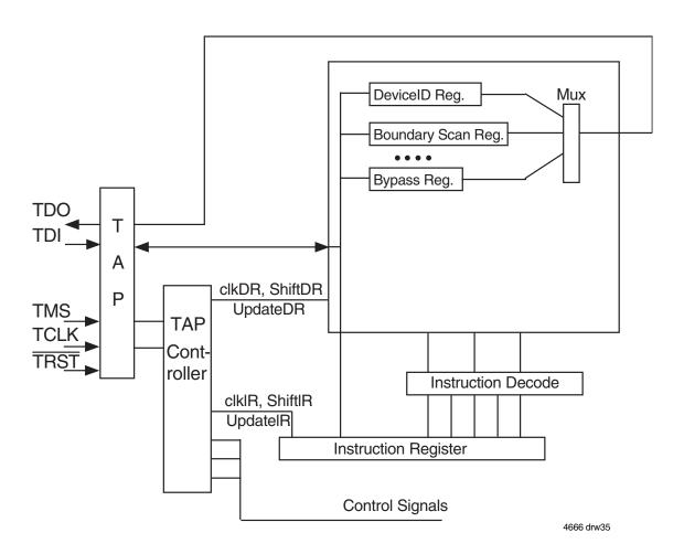
Figure 32. Boundary Scan Architecture
