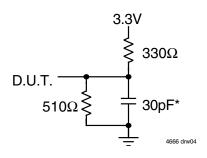
Figure 2a. Output Load
