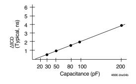
Figure 2c. Lumped Capacitive Load, Typical Derating
