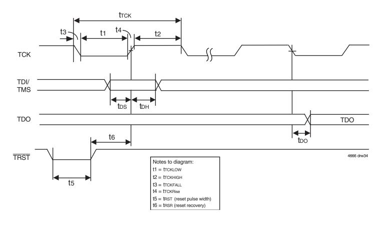
Figure 31. Standard JTAG Timing
