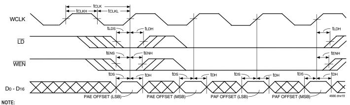
1. This diagram is based on programming the IDT72V293 x18 bus width. Add one extra cycle to both the PAE offset and PAF offset for x9 bus width.
