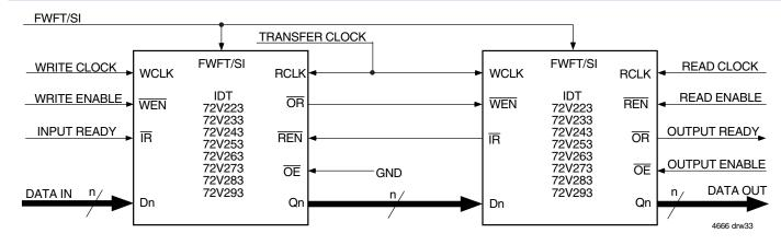
Figure 30. Block Diagram of Depth Expansion
