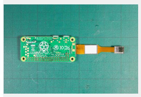
Peel the small piece of plastic film off the camera lens, and then place the camera lens into the large hole on the OctoCam mount, as in the image below.
