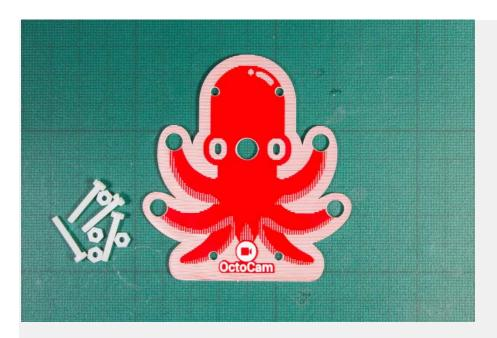
Let's start by taking the red OctoCam mount, the four bolts and four of the nuts. Push each of the four bolts through the circular holes at the top and bottom of the mount, from the front.
