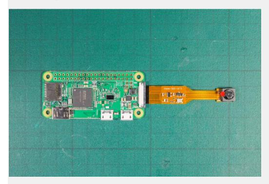
Now flip the Pi Zero W with connected camera over. Peel the paper off the sticky tape on the back of the camera module (just the one on the camera module itself). Take the small rubber foot and stick the non-sticky side of it to the sticky tape on the camera module, so that the sticky side of the rubber foot is exposed. This means that when you mount the camera, the sticky side of the rubber foot will stick to the back of the Pi Zero W, holding it in place.
