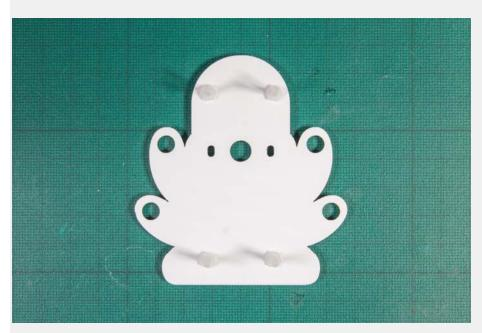
Take the four spacers and slip them onto each of the four bolts. They will space the camera just the right distance away from the Pi Zero W, and the rubber foot (that we'll add later) will prevent too much heat from radiating from the Pi Zero W's CPU to the camera.
