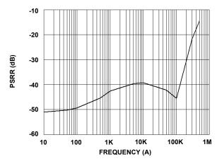
FIGURE 10. LDO1 POWER SUPPLY REJECTION (IOUT1 = 100mA, COUT = 10µF CERAMIC)
