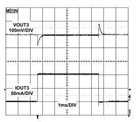
FIGURE 5. LDO3 LOAD TRANSIENT RESPONSE (10mA to 100mA)
