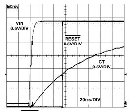
FIGURE 7. RESET DELAY DURING START-UP (CT =  $0.01\mu$ F)
