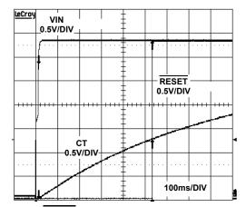
FIGURE 8. RESET DELAY DURING START-UP (CT =  $0.1\mu$ F)
