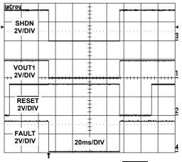
FIGURE 6. SHUTDOWN FAULT AND RESET OPERATION
