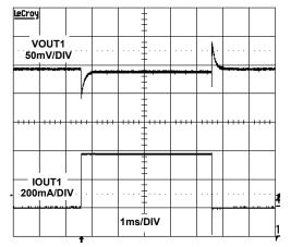
FIGURE 3. LDO1 LOAD TRANSIENT RESPONSE (10mA to 380mA)
