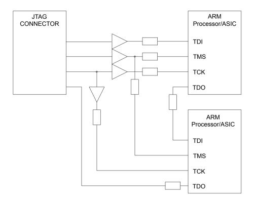
Figure 2-11 JTAG connection with de-skewed buffers
