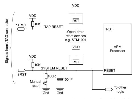
Figure 1-1 Example reset circuit logic
