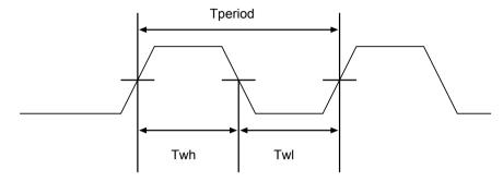
Figure 2-5 Clock waveforms
