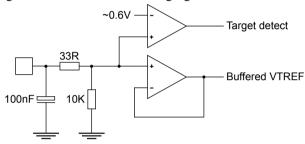
Figure 2-18 VTRef input (decoupled)
