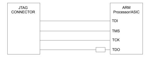
Figure 2-7 JTAG connection without buffers
