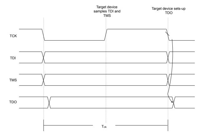
Figure 2-6 JTAG port timing diagram
