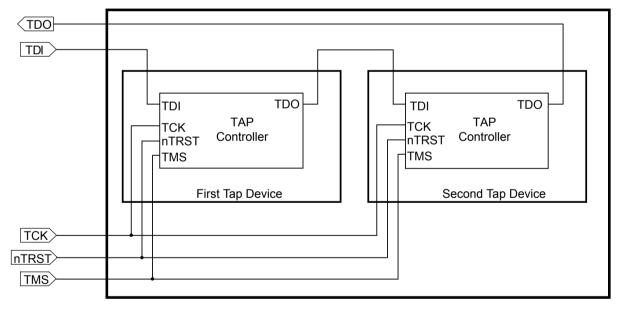
Figure 1-2 TAP Controllers serially chained within an ASIC
