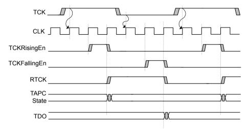
Figure 5-4 Timing diagram for the D-type JTAG synchronizer
