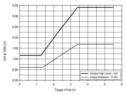
Figure 1-4 Target interface logic levels
