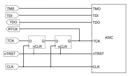
Figure 5-1 Basic JTAG port synchronizer
