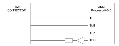
Figure 2-8 JTAG connection with TDO buffer
