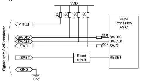
Figure 2-3 Typical SWD connections
