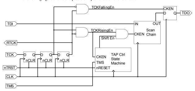
Figure 5-3 JTAG port synchronizer for single rising-edge D-type ASIC design rules
