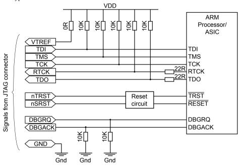
Figure 1-3 Typical JTAG connection scheme
