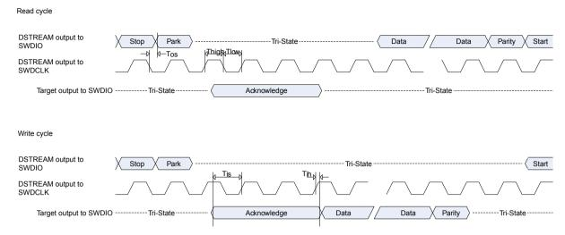
Figure 2-4 SWD timing diagrams
