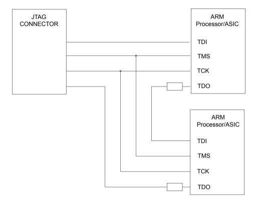
Figure 2-9 Daisy-chained JTAG connection without buffers
