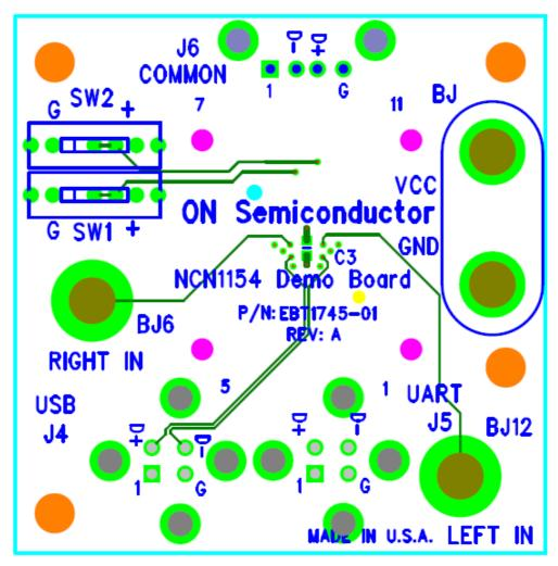
Figure 4. Bottom Layer Routing
