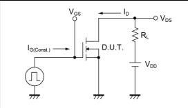
Fig.3-1 AVALANCHE MEASUREMENT CIRCUIT
