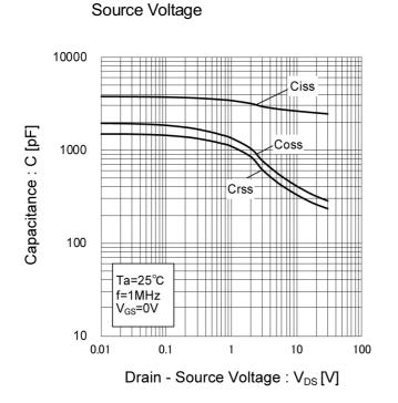
Fig.17 Typical Capacitance vs. Drain -
