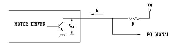
CAUTION: THE RD SINGAL LEAD WIRE MUST BE KEPT AWAY FROM "+" LEAD WIRE & "-" LEAD WIRE.
